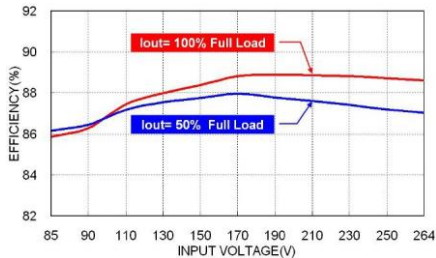
Efficiency vs. Input Voltage M□D40UT63M6B
