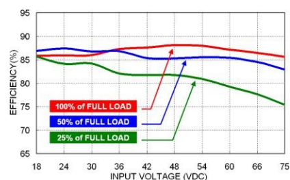
PDL12-48S05W Efficiency vs. Input Voltage
