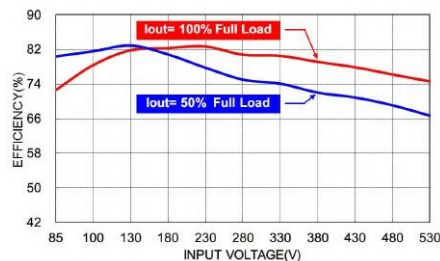
PSC06HS24B Efficiency vs. Input Voltage
